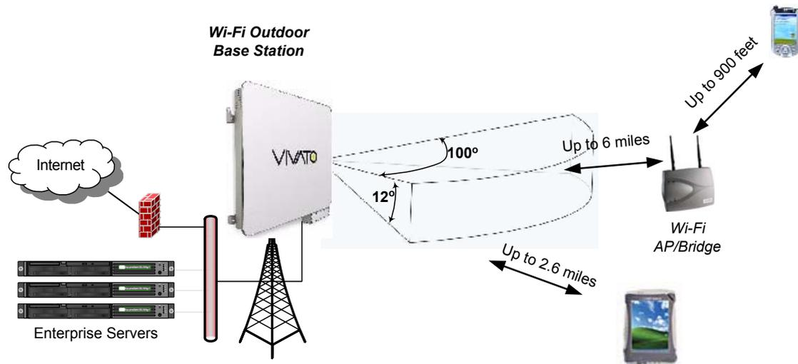
**Figure 1 Long Range High Coverage Wi-Fi**
