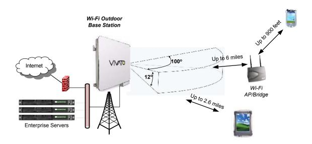
Figure 1 Long Range High Coverage Wi-Fi
